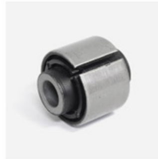
BUSH-UPR SUSPENSION ARM Model No : 55118-3R000 / 55130-C1100 Cars : HYUNDAI YF SONATA / LF SONATA
